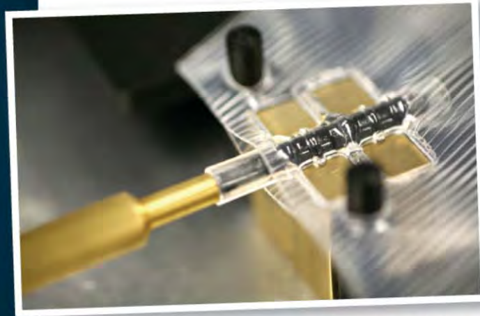
<< Illustration 3: Using the established ecoGenesis welding process, it is now possible to switch a PVC media reservoir bag, being mandrel-welded using a Teflon-coated tooling setup, to TPE. >>
